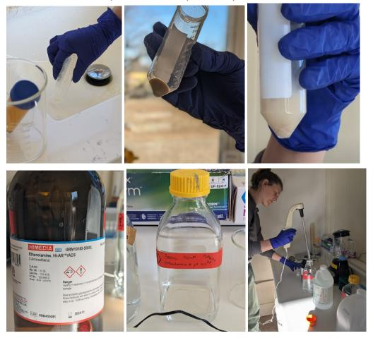
4. Wash the tube three times with 20mL of 150mM ethanolamine, pH10.5 and pour into the blender and blend (90mL) for 2 minutes on low speed.
